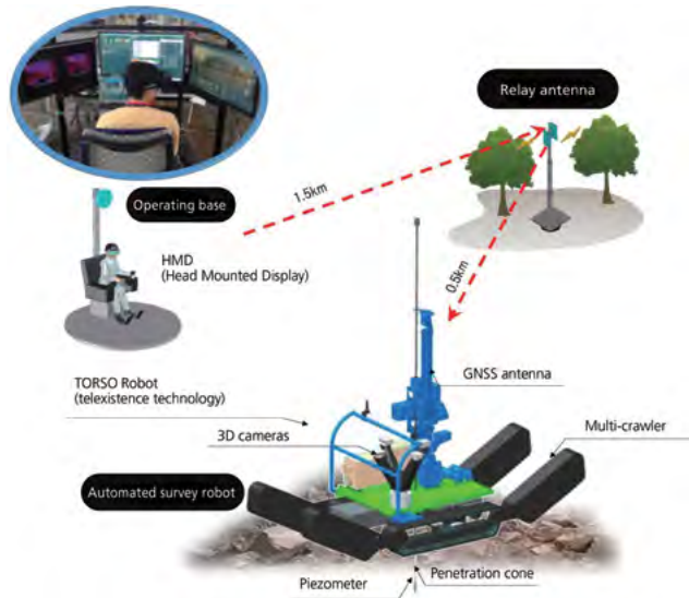
(Above) Installation of a relay antenna allows for remote operation up to about 2 km from the operating base
