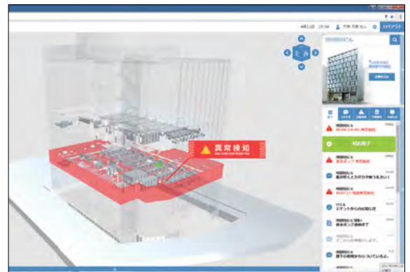
The system shows the position of a detected irregularity on the screen
