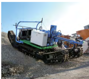
(Above) Installation of a relay antenna allows for remote operation up to about 2 km from the operating base
