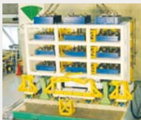
Tri-axial shaking table for developing anti-seismic technologies
