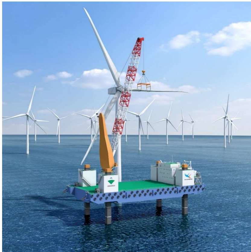
Project 05 SEP (Self Elevating Platform) Image
