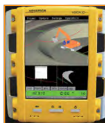
Operating construction machinery using an MG monitor (photo to the left) enables very accurate work
