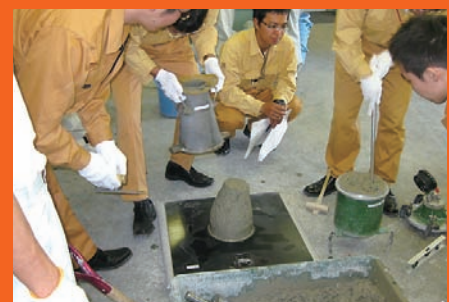
Practicing Concrete Test (Slump and Air Content *2 )
