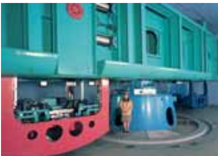
Geotechnical Centrifuge System Experimentally simulates ground movement using a scale model
