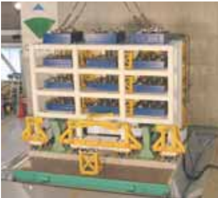
Tri-axial Shaking Table Capable of simulating earthquakes twice the magnitude of the 1995 Kobe Earthquake
