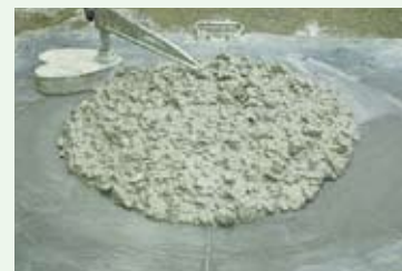
Testing the fluidity of Obayashi's new concrete
