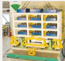
Tri-axial shaking table for developing anti-seismic technologies
