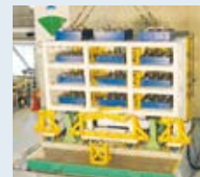
Tri-axial shaking table for developing anti-seismic technologies
